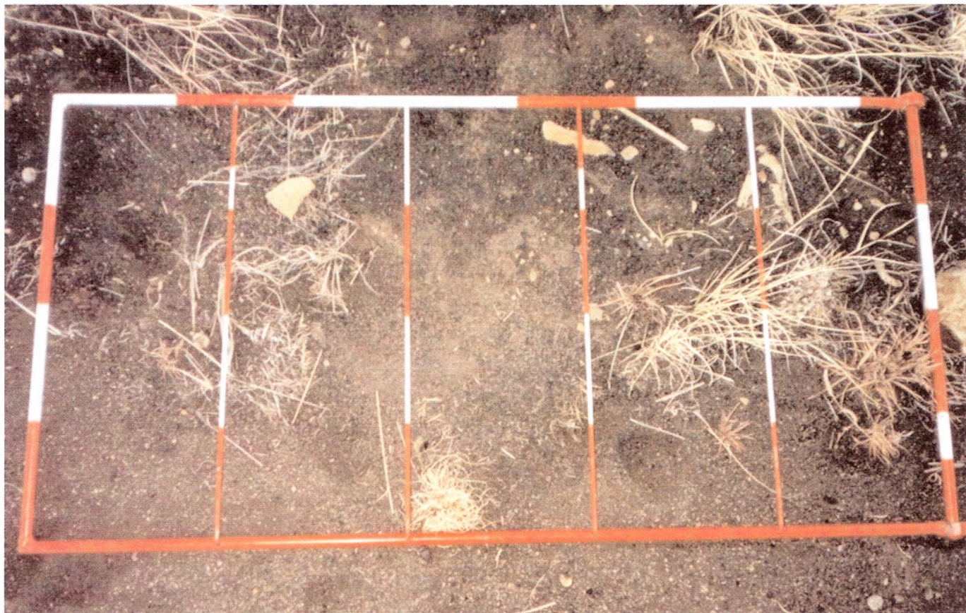
Figure 2. In the field illustration of the Daubenmire method plot arranged within the painted frame that designates area percentages. Each cross bar is removable for easy placement of the frame.
