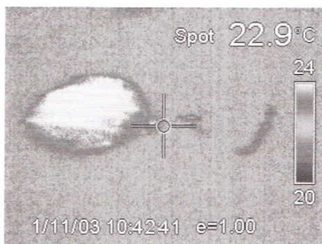
Figure 5. Thermal image of a weight thrown from right to left. The partial triangle image represents the impact of the weight handle.
